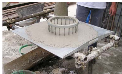
Fig. 4, 5, 6 - slump-flow, j-ring, V-funnel test.
